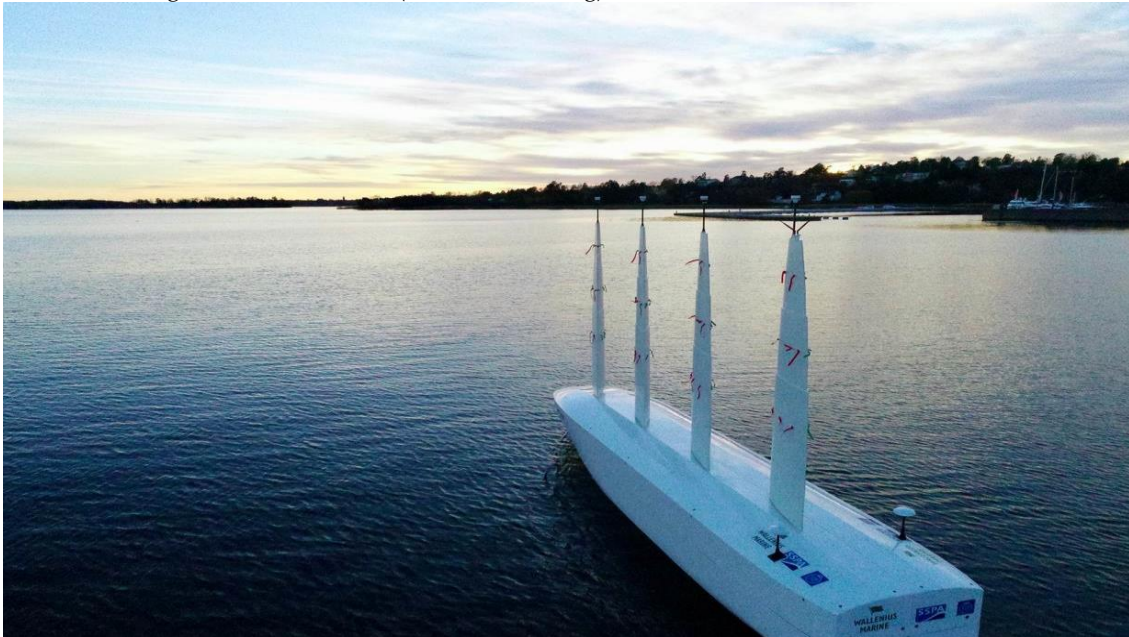
Figure 13. Scale model (seven metres long) of Oceanbird under test in the Baltic.
