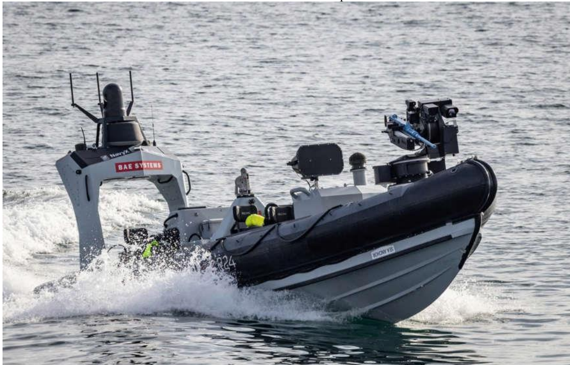
Figure 11. © UK Ministry of Defence. The PAC 24 Rigid Inflatable Boat (RIB) moves without a human driver present.
