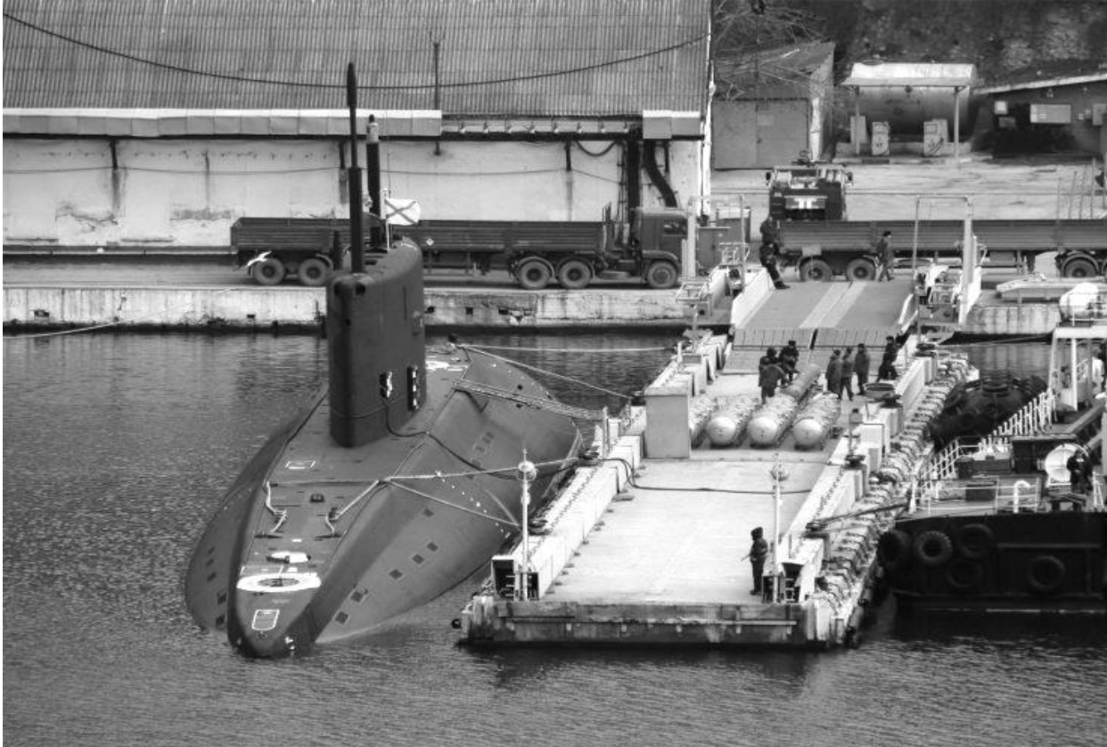
Figure 10. Kalibr missiles are being loaded onboard the Kilo-class submarine Velikiy Novgorod (IBT 2022).
